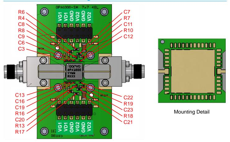
RF Layer is 0.008" thick Rogers Corp. RO40003C ( $\epsilon r = 3.35$ ). Metal layers are 0.5 oz. copper. The microstrip line at the connector interface is optimized for the Southwest Microwave end launch connector 1092-02A-5.
